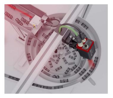
The VISOR® **XE** Object Al's classification detector reliably distinguishes even very similar-looking springs, ensuring accurate feeding to the machine. By providing just a few examples for each class, the classifier automatically learns to differentiate between types.
