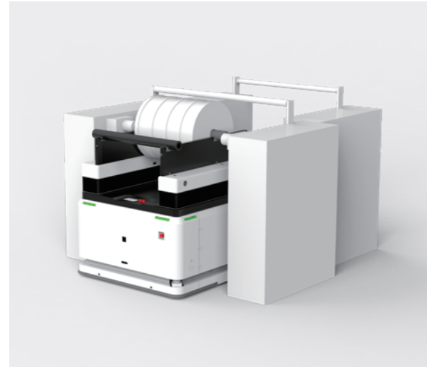
High-precision docking of AMRs to coating CMRs
