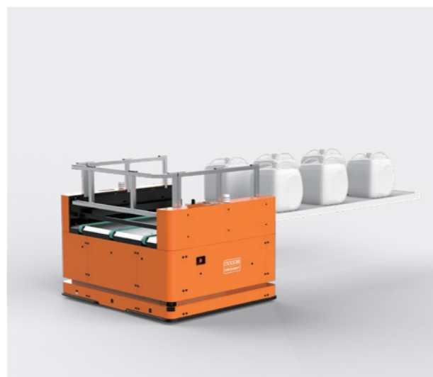
Conveyor / Buffer conveyor docking
