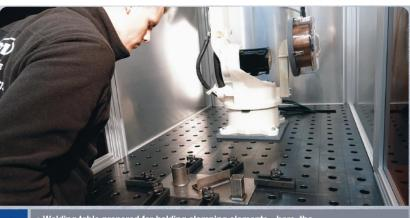
**3** • Welding table prepared for holding clamping elements - here, the operator is shown during the mounting phase
