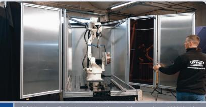
Safety housing with aluminum sheet reinforcement, large opening and foldable side elements - seen here in setup mode
