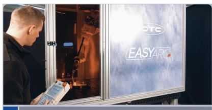
Automatic welding process with the machine closed operator observes the process through the safety windows
