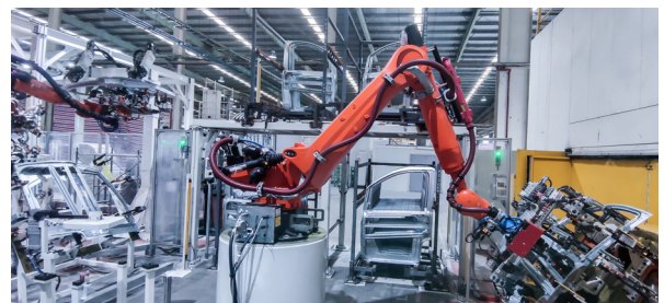
Vision-Guided Car Door Inner Panel Picking
