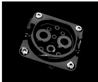
Car charging port
