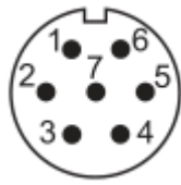
Figure 6-14 EtherCAT debug interface
