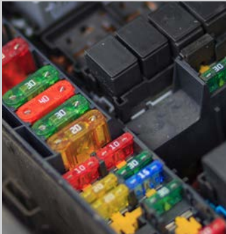
Inspection of car fuses – color and material
