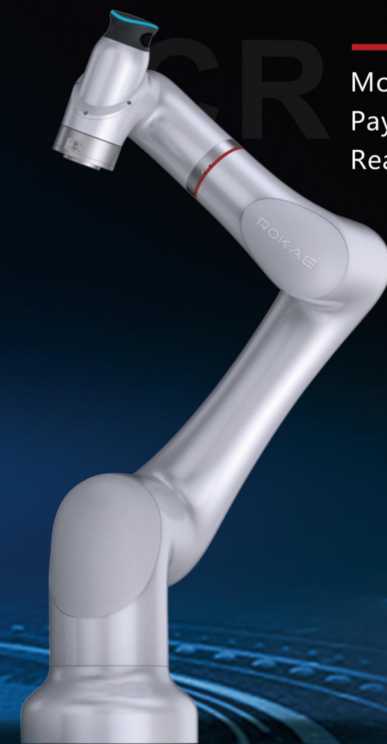
Model CR20 Payload 20kg Reach 1,798mm
