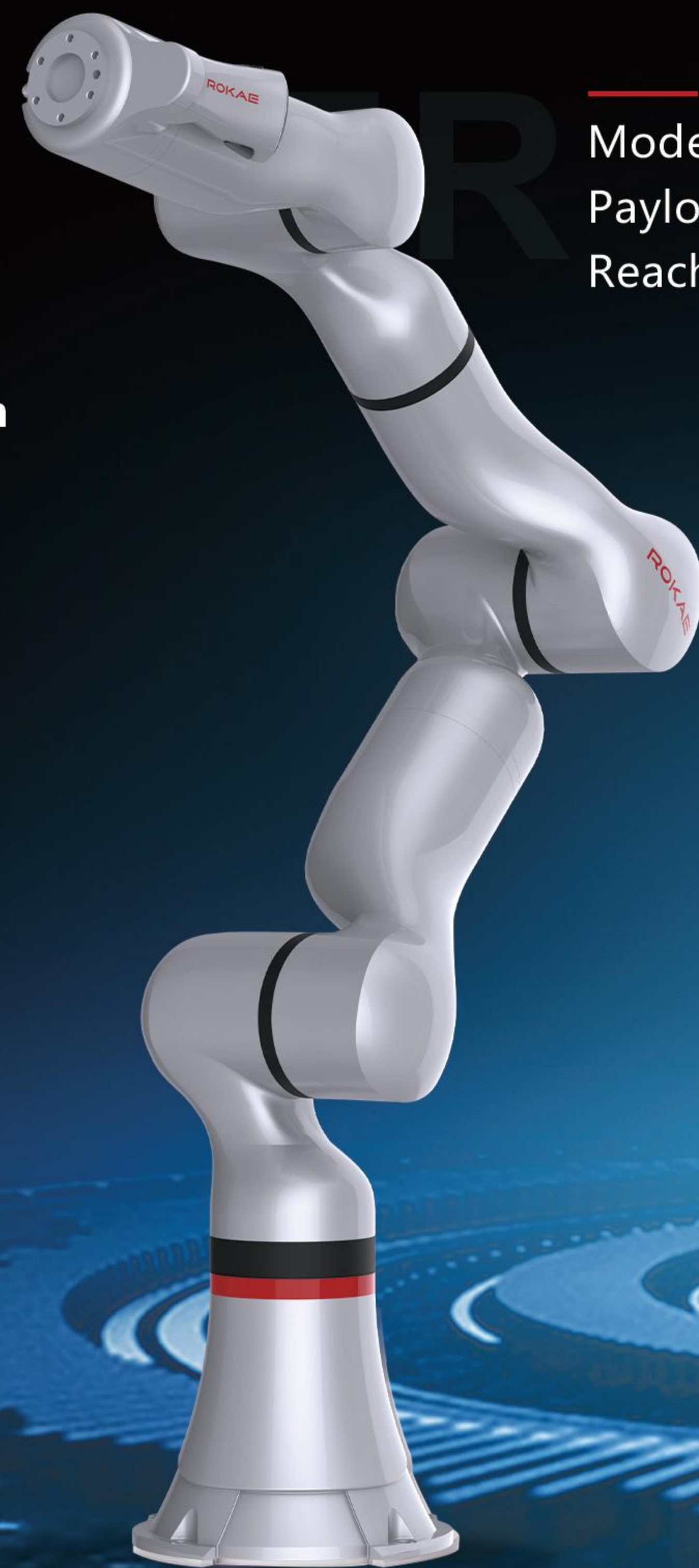
Model ER7 Payload 7kg Reach 1,125mm
