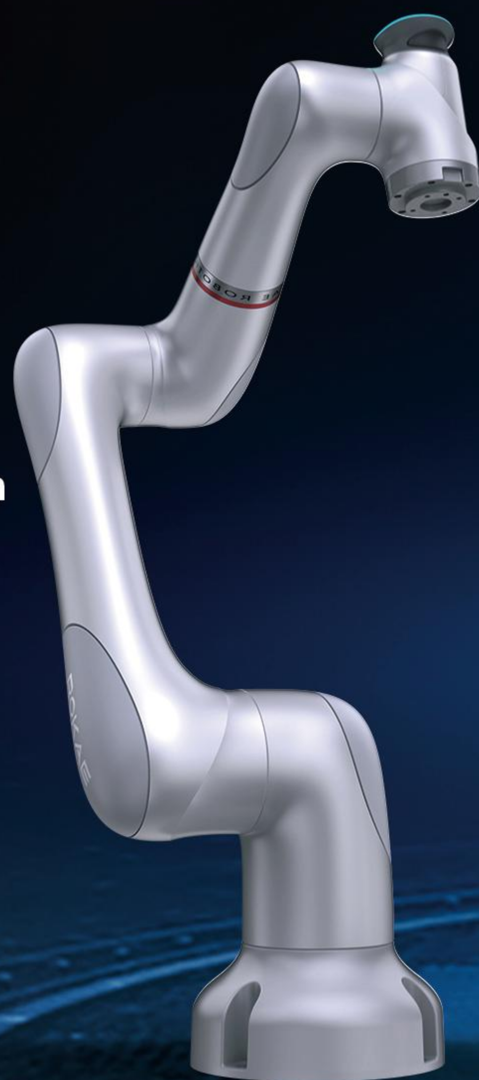
CR Model CR7 Payload 7kg Reach 988mm
