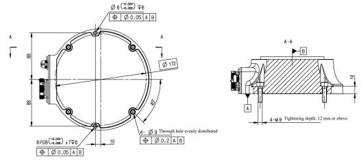
Put pins in the reserved cylindrical pin holes for accurate positioning. Then use four M8×30 hexagon socket head cap screws (strength grade 12.9) to fix the robot's base on the bracket.
