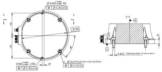
Put pins in the reserved cylindrical pin holes for accurate positioning. Then use four M12×40 hexagon socket head cap screws (strength grade 12.9) to fix the robot's base on the bracket.
