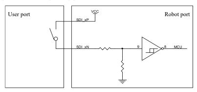
The principle of both loops is the same, and 24 VDC signals are supported.
