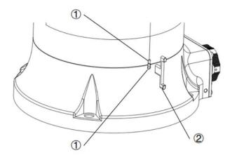
Step 2: Calibrate axes 2, 3, 5, and 6
