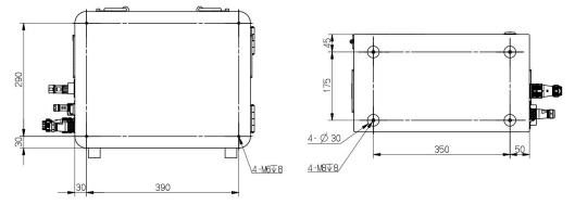
There are four M6 threaded holes in 8 mm depth on the back of the control cab and four M8 threaded holes in M8 depth at the bottom. The fixing mode shall be chosen according to the operating environment.
