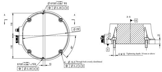
Put pins in the reserved cylindrical pin holes for accurate positioning. Then use four  $M12 \times 40$  hexagon socket head cap screws (strength grade 12.9) to fix the robot's base on the bracket.
