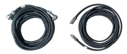
Connect the socket marked with the "ROBOT POWER" on the side of the control cab with the socket marked with ① at the manipulator base using a power relay cable, and connect the socket marked with the "ROBOT SIGNAL" on the side of the control cab with the socket marked with ② at the manipulator base using a signal relay cable.
