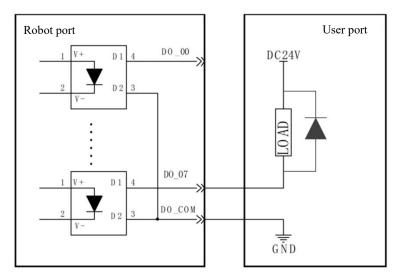
When the output is active high, the DO\_COM (common port) is connected to 24 VDC, as shown below.
