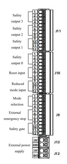
Each group of safety input or safety output signals is dual-channel redundant, so each group contains two inputs/outputs, namely "Loop 1" and "Loop 2", with a total of 4 terminals. Definition of pins:
