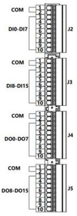
The control cab is equipped with 16 general-purpose digital inputs and 16 general-purpose digital outputs as standard, with pin definition as follows:
