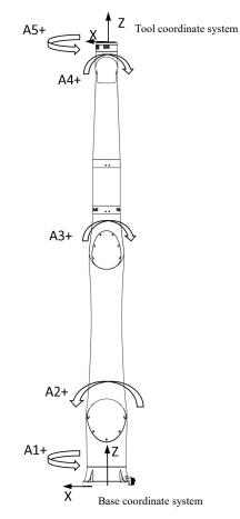
forward rotation in the +Y direction, and the A3 and A4 perform forward rotation in the -Y direction.
